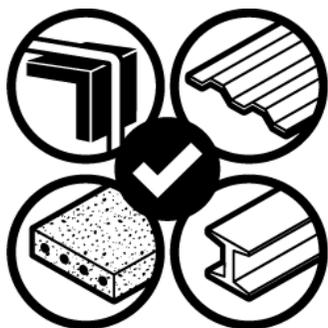
Additionally, while the ANSI Z359.14- 2021 (Class 2) standard does not address edges other than steel, the V-SHOCK EDGE SRL has been tested using the methods in ANSI Z359.14-2014 with the following edges:
